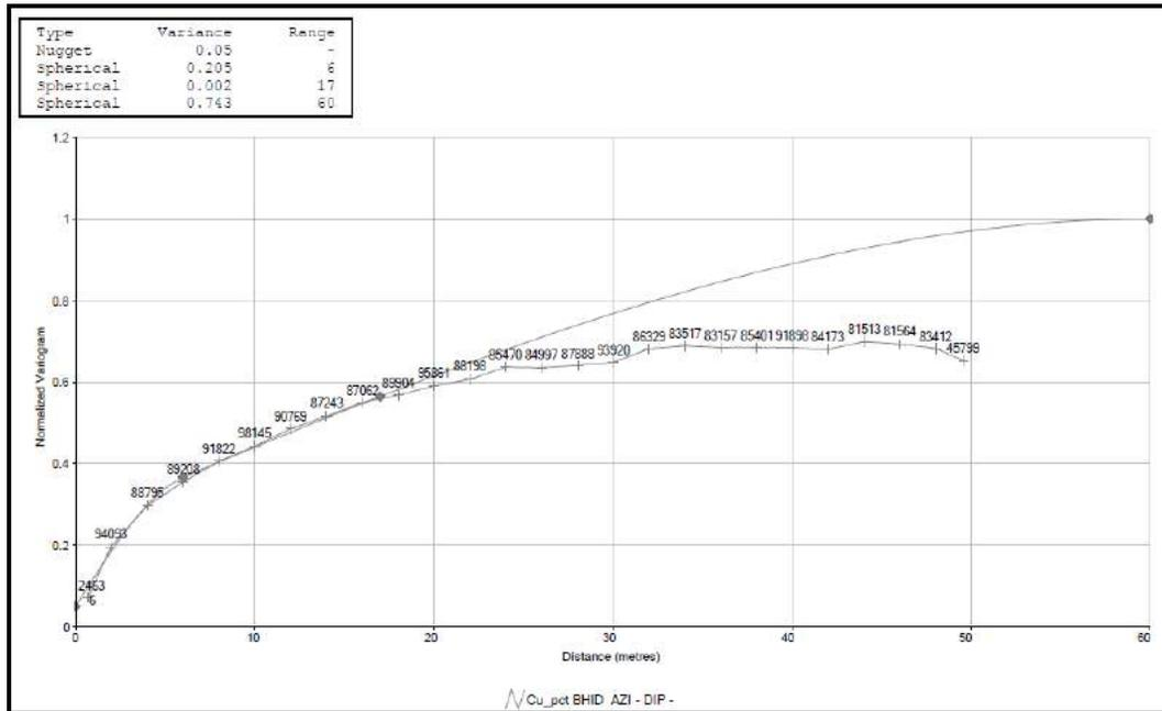
Figure 14.8 Copper Downhole Variograms for Zone 1 (Hypogene Mineralization)
